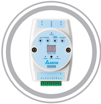
The Tracker Gateway Unit (TGU) is the device used as a converter between MODBUS RS485 and MODBUS TCP communication protocols.
